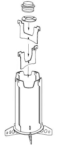
The insert with Trangia spirit burner is quickly assembled and ready for use.
